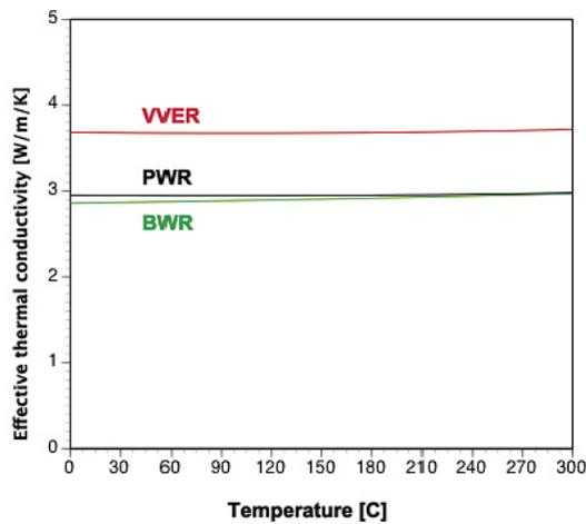
Figure 6-20. Effective thermal conductivity of the fuelled area in the longitudinal direction.
