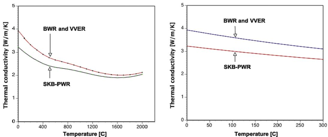
**Figure 2-5.** Thermal conductivity of the spent fuel pellets (MATPRO 2014).
