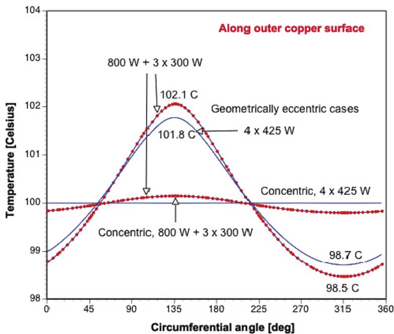
Figure 7-2. Temperature variation in the circumferential direction of the external copper wall in different cases.
