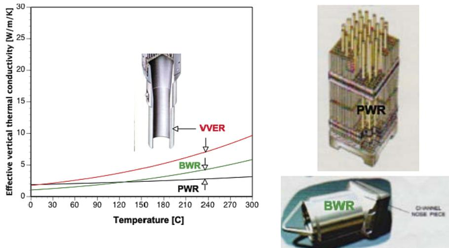
**Figure 6-22.** Effective thermal conductivity of fuel assembly bottom end structure in longitudinal (vertical) direction.
