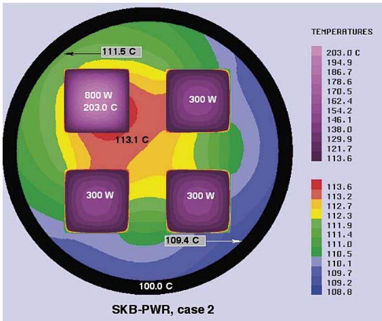
Figure 5-9. Temperatures inside the SKB-PWR fuel canister in case 2.
