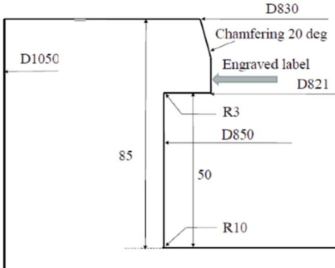
**Figure 6-10.** Canister copper lid. The dimensions reflect the geometry before welding deformations. Also the location of the engraved canister identification label is shown in the figure (Raiko 2012, Figure 15).
