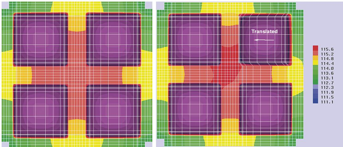
**Figure 7-7.** Enlargements of the central area of the Posiva-BWR canister (12 fuel assemblies) in reference case 0, showing the temperature distributions of the case in which all fuel assemblies are concentric in the compartment steel tubes (left) and in which one fuel assembly is moved to the left against the edge of the steel tube (right).
