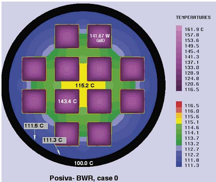
Figure 5-3. Temperatures inside the Posiva-BWR fuel canister in reference case 0.
