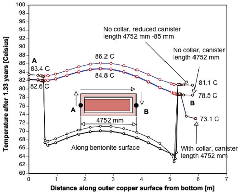
Figure 6-12. The effect of modelling the collar in the upper end of the canister.
