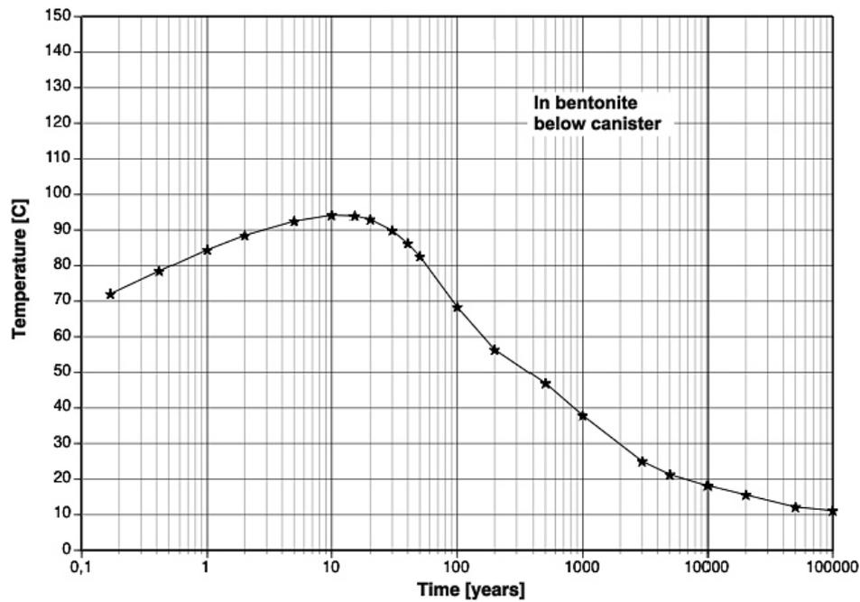
Figure 6-27. Evolution of the maximum bentonite buffer temperature in a SKB-BWR and PWR repository case (Hökmark et al. 2010).
