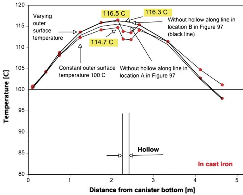
Figure 7-9. Longitudinal temperature profiles of the cast iron of the Posiva-BWR canister.
