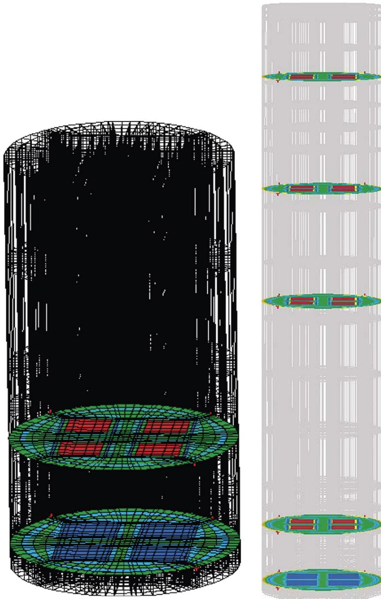
Figure 6-23. Visualization of the material types in the SKB-PWR canister.
