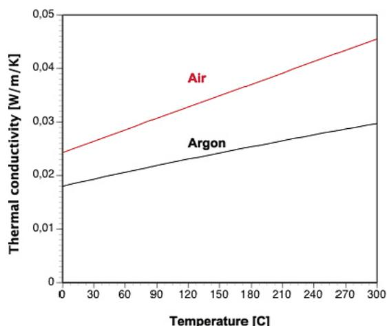
Figure 2-6. Thermal conductivity of argon (MATPRO 2014) and air (Fletcher 1991) at atmospheric pressure.
