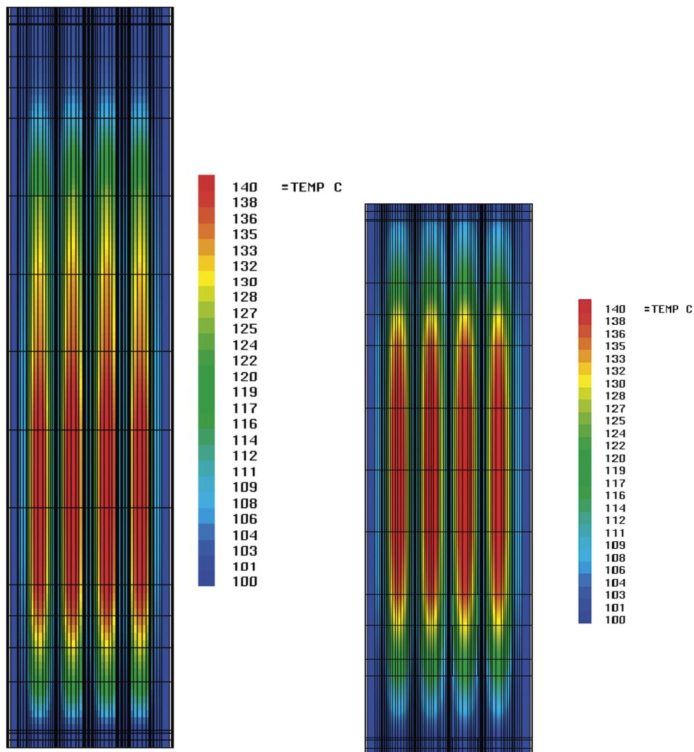
**Figure 6-34.** Left figure: temperature distribution of the Posiva-BWR-type canister in the longitudinal cross section passing through the centres of the fuel assemblies. Right figure: Posiva-VVER-type canister.
