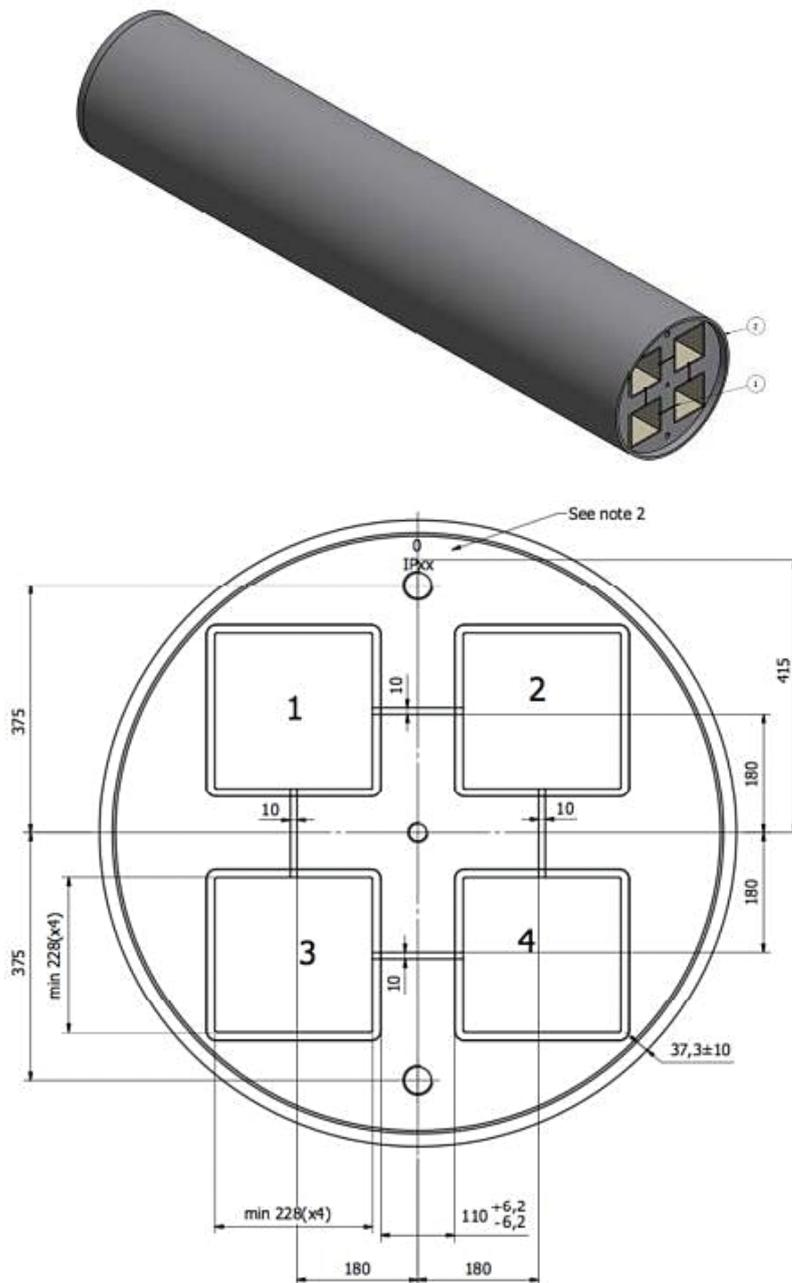
**Figure 2-3.** Cross-sectional dimensions of the SKB-PWR canister insert. The current specified minimum size of the compartment channel is 229.9 x 229.9 mm.
