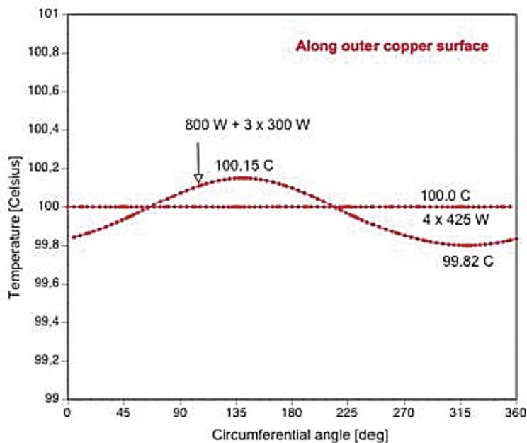
Figure 6-16. Temperature variation in the circumferential direction along the external copper wall. Temperature distributions in the case of  $800\text{ W} + 3 \times 300\text{ W} = 1700\text{ W}$  (left) and in the case of  $4 \times 425\text{ W}$ .
