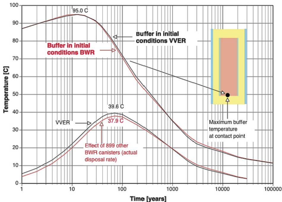
**Figure 6-26.** Maximum temperature evolution in the bentonite buffer of the Posiva-BWR canister (the spacing is 8.9 m) and of the Posiva-VVER canister (the spacing is 7.5 m). Contribution of the other canisters in a repository panel is summed in the curves. Upper curves also include initial ambient rock temperature of 10.5 °C of Olkiluoto repository. Lower curves give the contribution of the other canisters in the repository.
