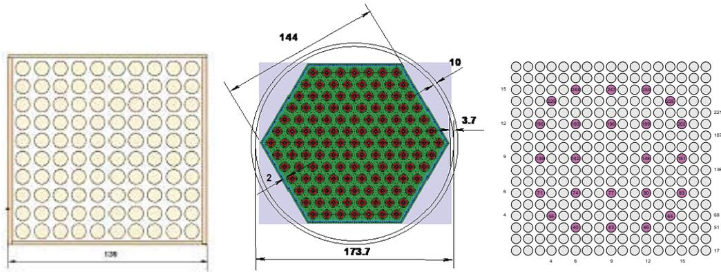
**Figure 2-4.** Posiva-BWR fuel assembly surrounded by the fuel channel (left), Posiva-VVER-440 fuel assembly cross section and surrounding steel tube (middle) and SKB-PWR fuel assembly (right). Figures are not in scale.
