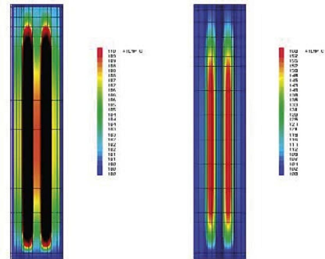
*Figure 6-35. Example of the temperature distribution of the SKB-PWR-type canister cross section. Two scales are used to better visualize the temperature of the cast iron (left) and of the fuel pellets (right).*
