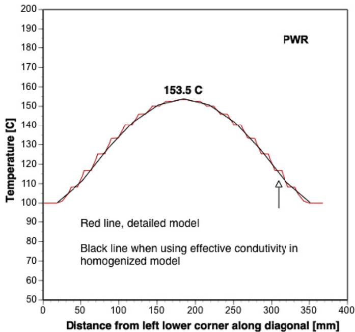
**Figure 4-10.** Temperature profile along a 45 degrees line through the SKB-PWR fuel rod array area. The temperature on the outer edges is 100 °C.
