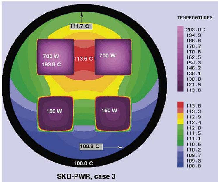
Figure 5-10. Temperatures inside the SKB-PWR fuel canister in case 3.
