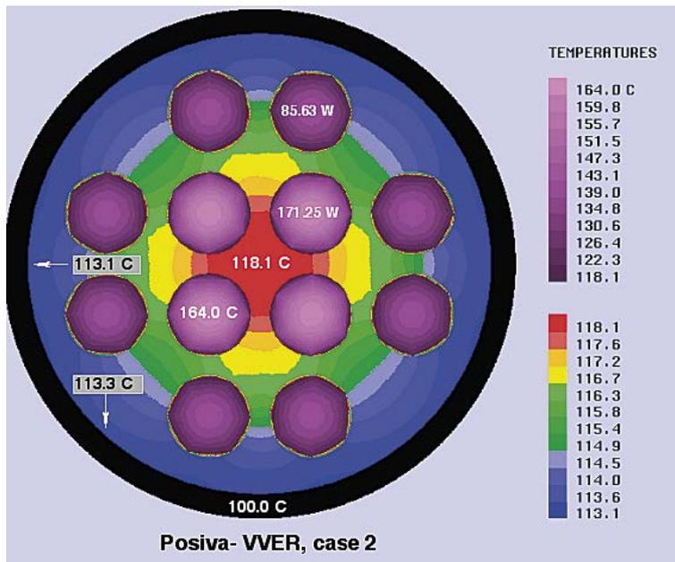
Figure 5-15. Temperatures inside the Posiva-VVER fuel canister in case 2.
