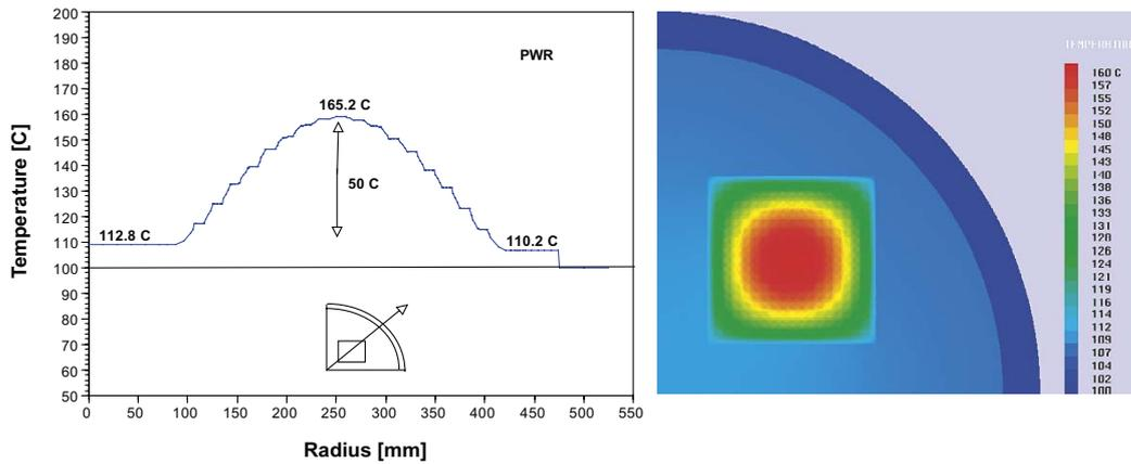
**Figure 4-4.** Temperature distribution along 45 degrees line in SKB-PWR canister. The radius denotes the distance from the centre of the canister.
