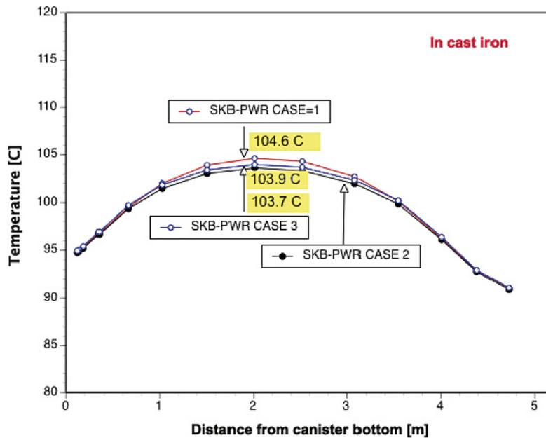
Figure 6-37. Temperature profile of the cast iron of the SKB-PWR canister after 10–12 years.
