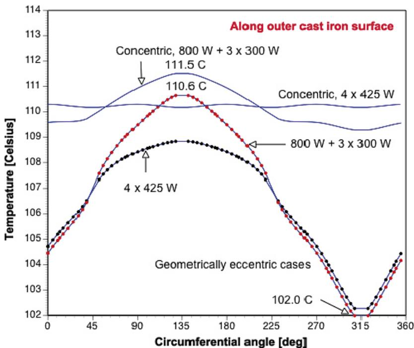
Figure 7-6. Temperature variation in the circumferential direction along the outer radius of the cast iron when the gap is closed on the opposite side for different cases.
