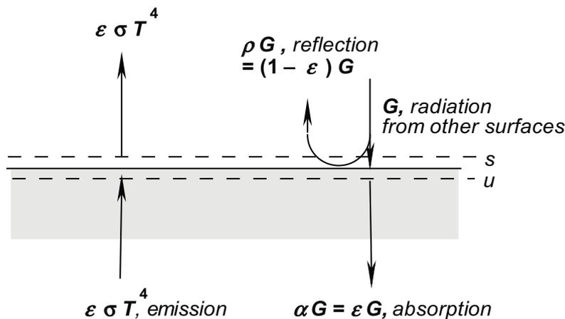
**Figure 3-2.** Thermal radiation near a grey surface. It is assumed that the emission and absorption coefficients of a surface are equal, i.e.,  $\varepsilon = \alpha$ .
