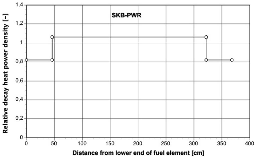
Figure 2-11. Decay heat power density distribution along the SKB-PWR fuel assembly length.
