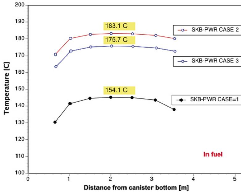
Figure 6-40. Temperature profile of the fuel pellets of the SKB-PWR canister after 1–2 years.
