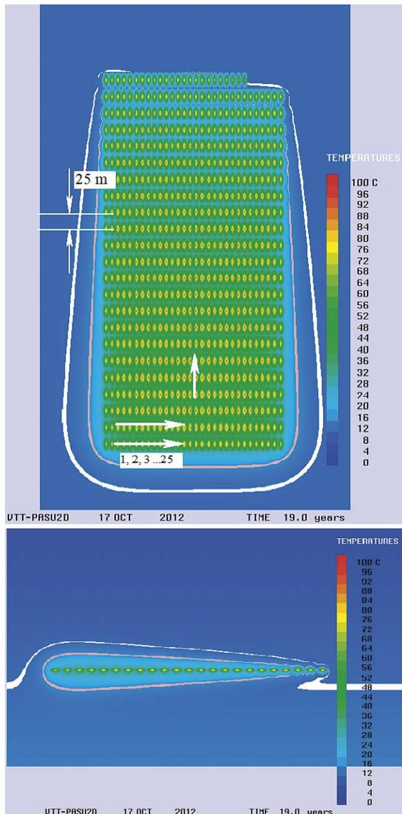
**Figure 6-25.** Temperature distribution of the repository in the horizontal cross-section (left) and in the vertical cross-section (right) after 19 years of operation, when the highest temperature of 95 °C is obtained on the hottest BWR canister surface. The tunnel spacing is 25 m, and the canister spacing is 8.9 m. The rate of canister deposition is 36 canisters per year.
