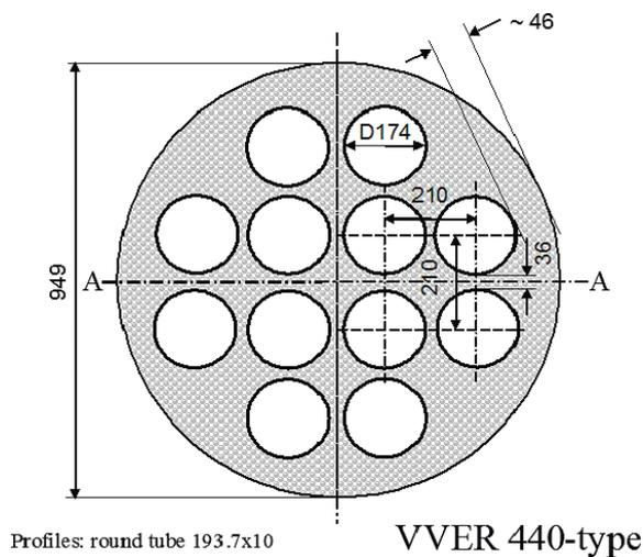
**Figure 2-2.** Cross-sectional dimensions of the Posiva-BWR and Posiva-VVER canister inserts (Raiko 2012).
