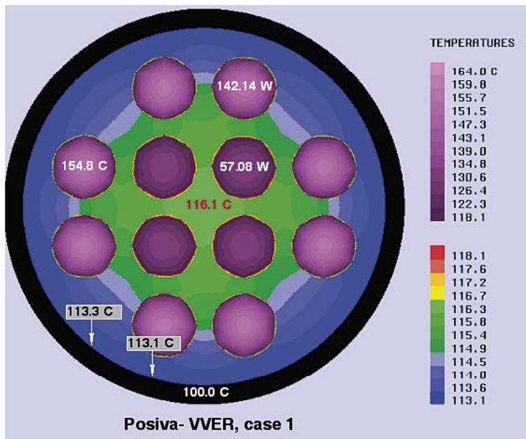
Figure 5-14. Temperatures inside the Posiva-VVER fuel assemblies in case 1.
