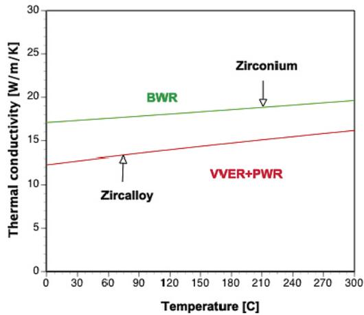
Figure 2-7. Thermal conductivity of zircalloy and zirconium (MATPRO 2014).
