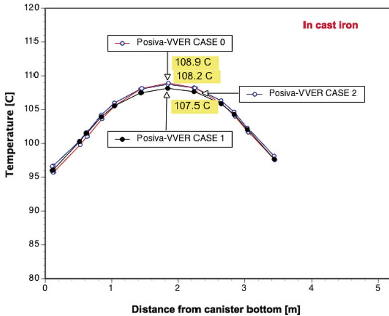
Figure 6-38. Temperature profile of the cast iron of the Posiva-VVER canister after 10–12 years.
