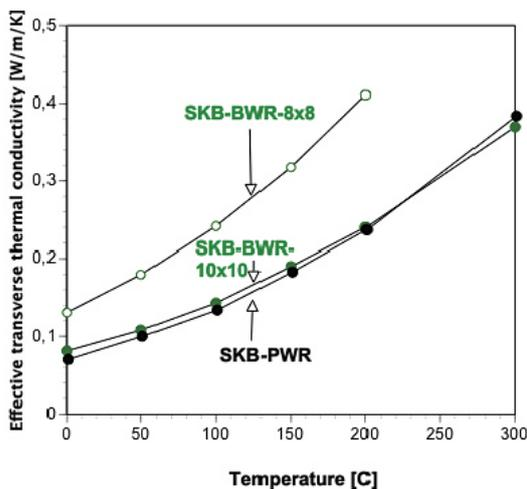
**Figure 4-12. Effective thermal conductivity of SKB-fuel rod arrays in the transverse (horizontal) direction.**
