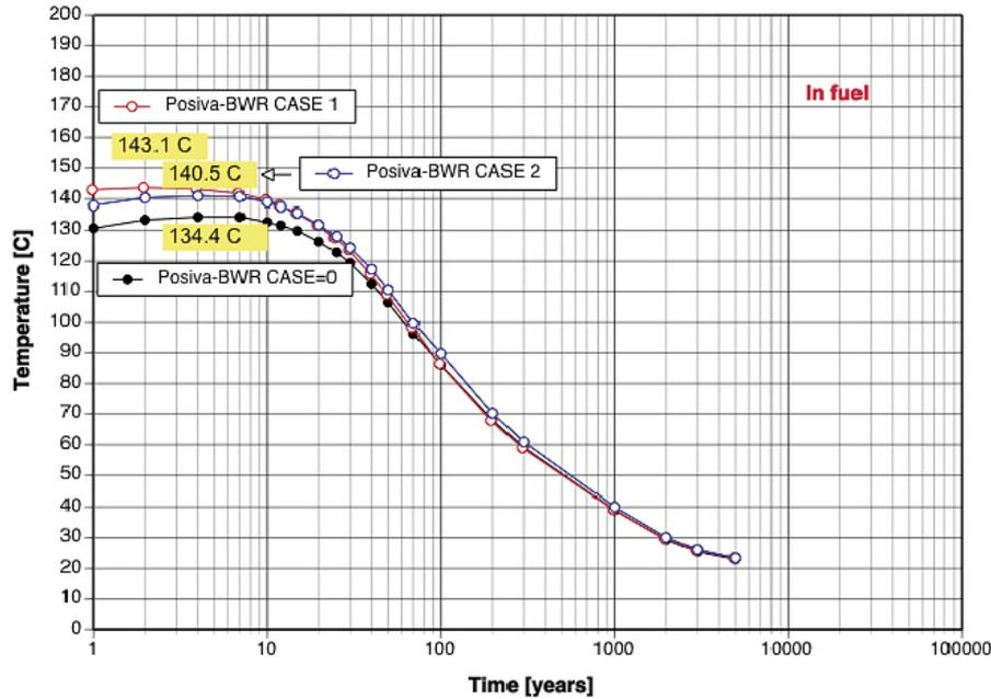
Figure 6-31. Maximum fuel pellet temperature evolution for the Posiva-BWR canister.
