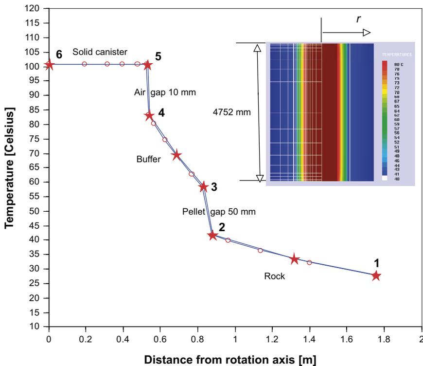
**Figure A-5.** Uniform heat generation in a homogenous cylinder.
