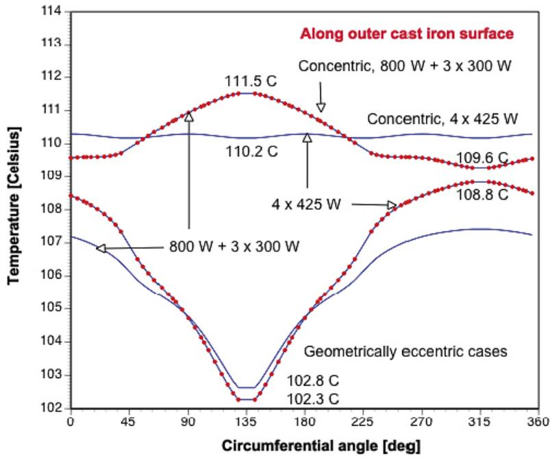
Figure 7-3. Temperature variation in the circumferential direction along the outer radius of the cast iron in different cases.
