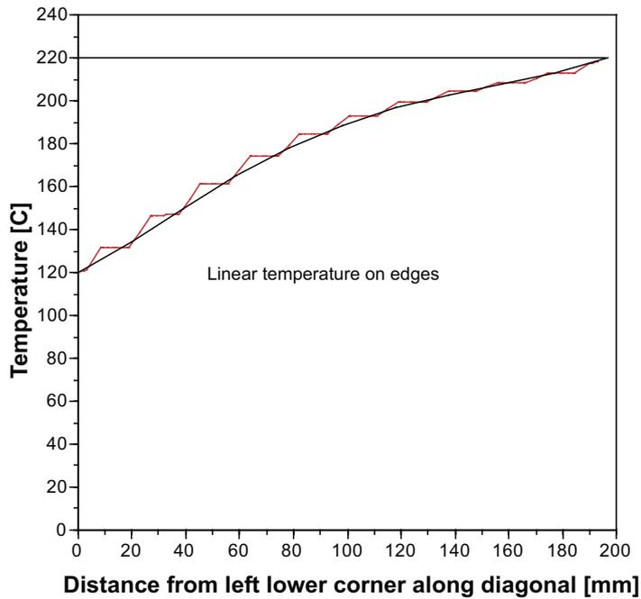
**Figure 4-8.** Temperature distribution along the diagonal starting from the lower-left corner and ending at the upper-right corner and passing through the BWR fuel assembly pellets.
