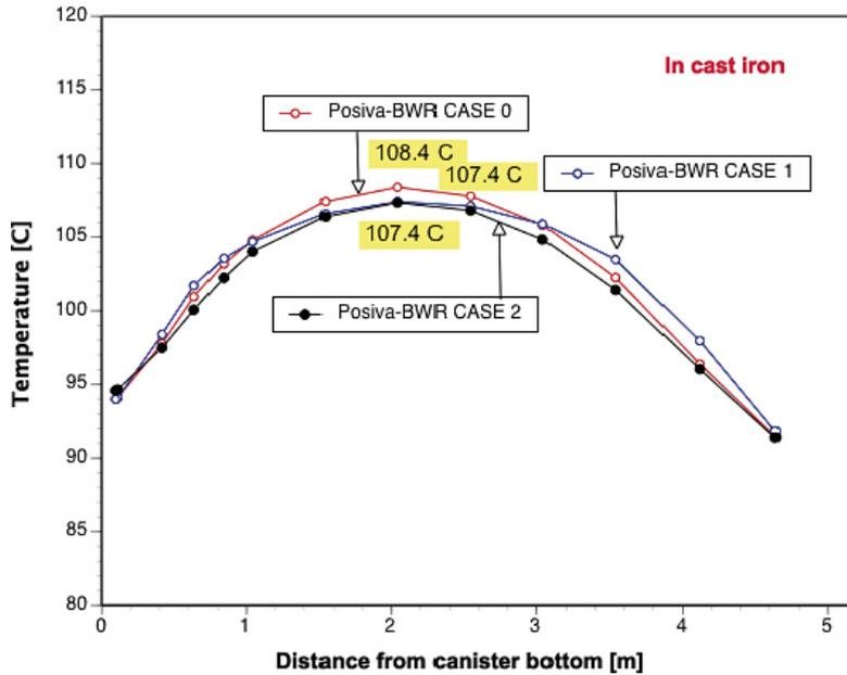
Figure 6-36. Temperature profile of the cast iron of the Posiva-BWR canister after 10–12 years.
