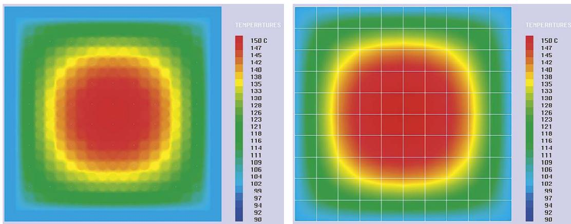
**Figure 4-9.** One SKB-PWR fuel assembly. On the left, the temperature distribution under the detailed model, and on the right, that under the homogenized fuel model. The maximum temperature in the middle is 153.5 °C.
