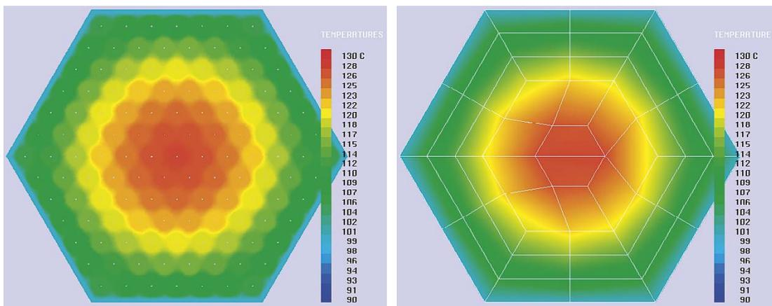
**Figure 4-11.** One VVER fuel assembly surrounded by a 2 mm zirconium fuel channel tube and analysed using a detailed model (left). The homogenized model only for the fuel rod array area (right). The temperature on the outer edges is 100 °C.
