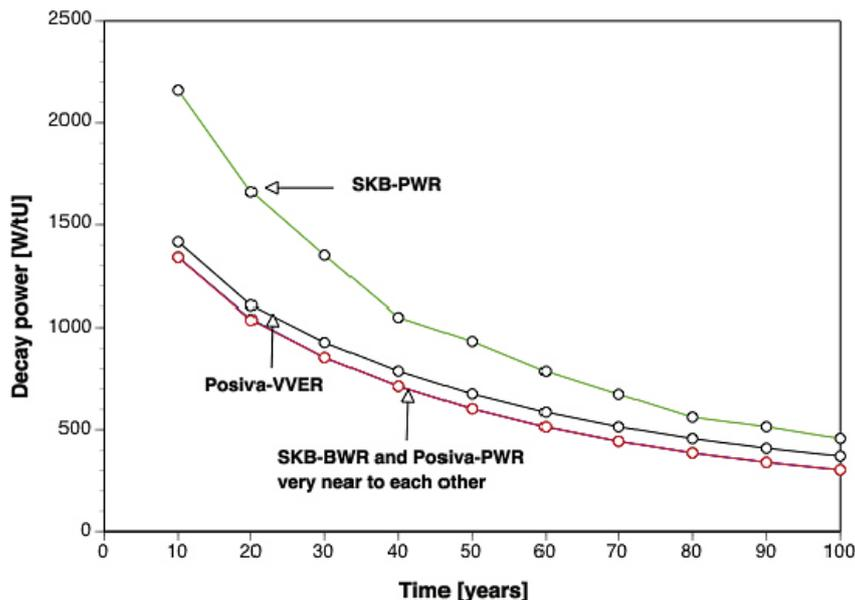
**Figure 2-9.** Decay heat power densities of the SKB-BWR and SKB-PWR spent fuel and of the Posiva-BWR and Posiva-VVER spent fuel. The cooling time is measured from the moment, at which the fuel is removed from a reactor. The decay heat is calculated for an equivalent ton of uranium in fresh fuel.
