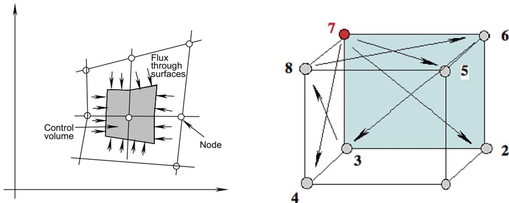
Figure 3-1. Heat fluxes to a planar control volume (left) and 8-node control volume (right).
