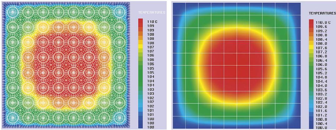
**Figure 4-13.** Detailed model of a SKB-BWR-8 × 8 fuel assembly (left) and the homogenized model (right). A fuel rod array surrounded by a zirconium fuel channel. In this case, in both models, the temperature of the outer edges is 100 °C.
