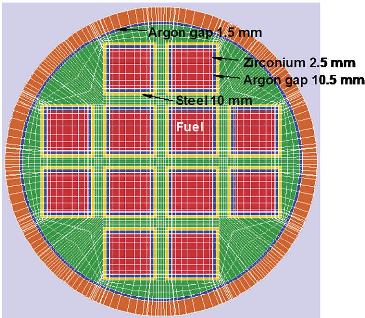
**Figure 5-2.** Materials of the homogenized 2D model of the Posiva-BWR fuel canister.
