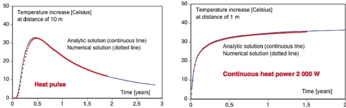
Figure A-2. Temperature evolutions in first verification case.
