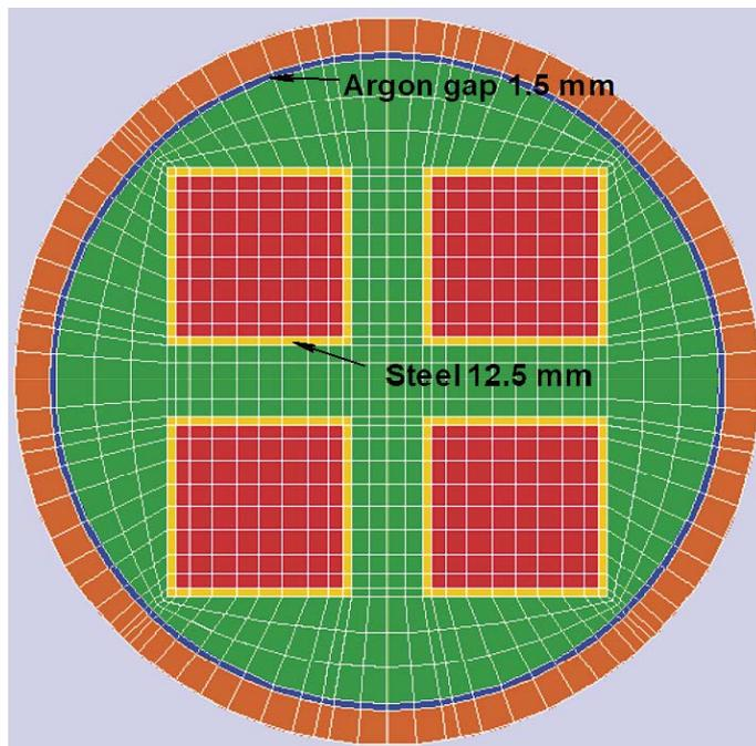
Figure 5-7. Materials of the homogenized 2D model of the SKB-PWR fuel canister.
