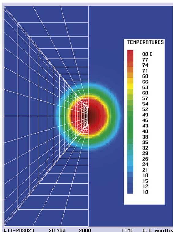
**Figure A-1.** Mesh and temperature distribution of a line heat source after  $\frac{1}{2}$  year.
