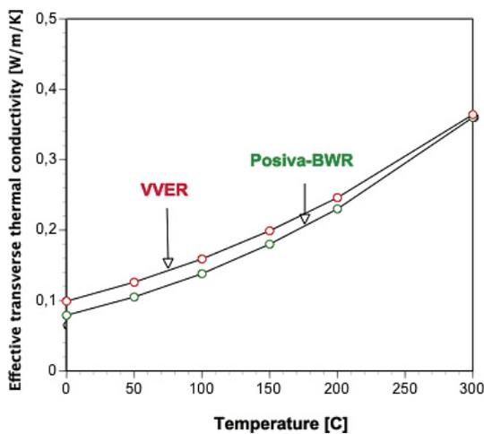
**Figure 4-14.** Effective thermal conductivity of Posiva-fuel rod arrays in the transverse (horizontal) direction.
