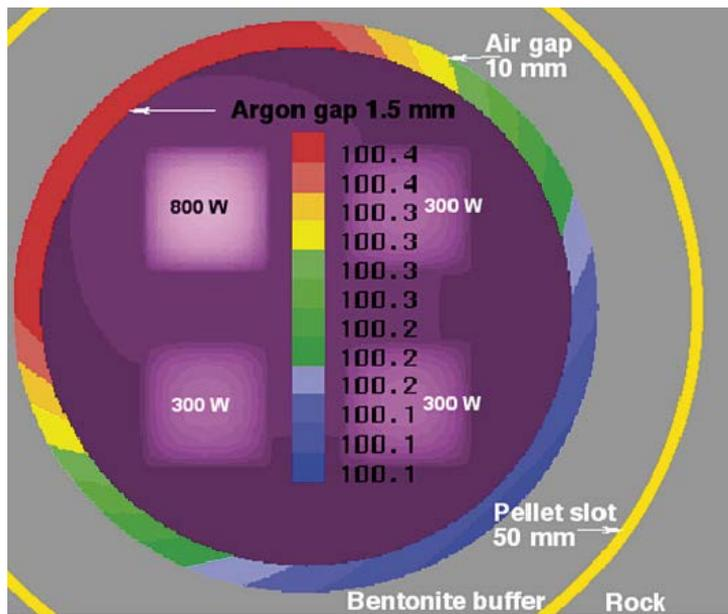
Figure 6-15. Asymmetric decay heat power of the SKB-PWR fuel assemblies.
