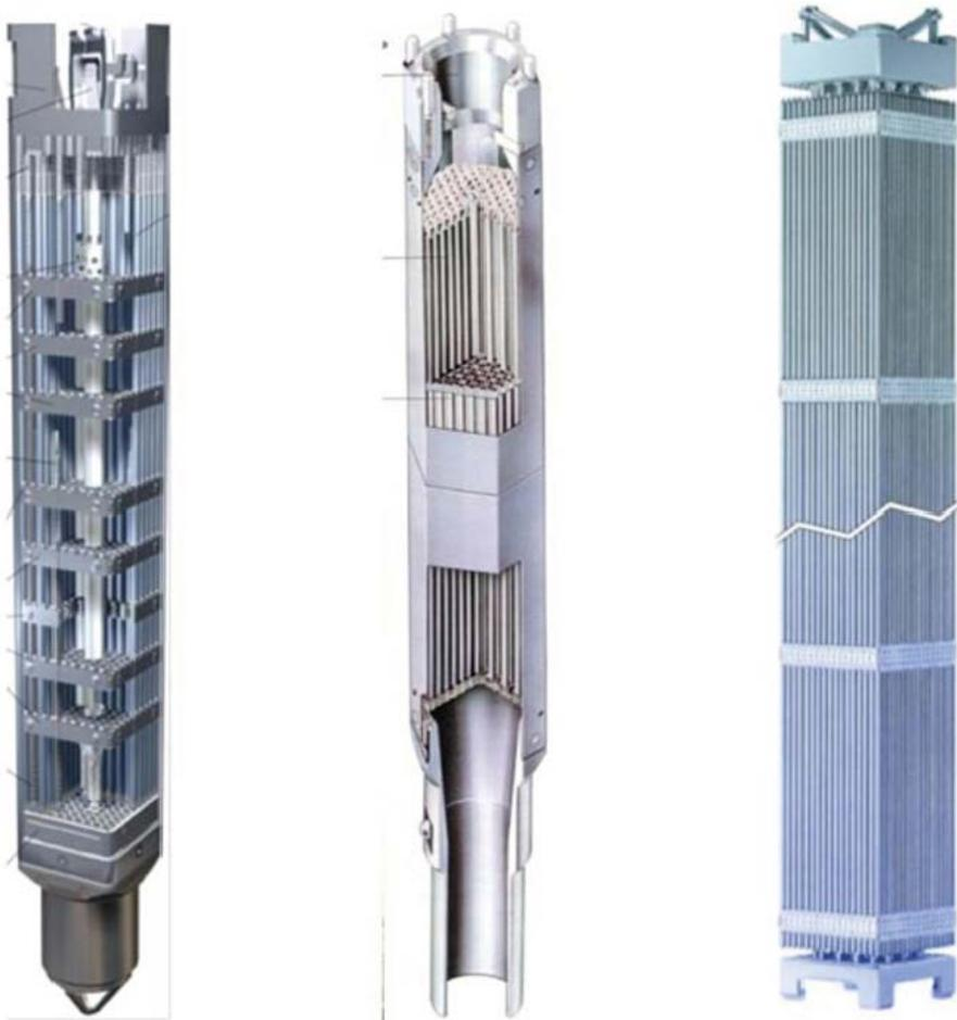
**Figure 2-1.** Schematic diagrams of partly cut-open BWR, VVER and PWR fuel assemblies (Raiko 2012). Figures are schematic and not in scale.
