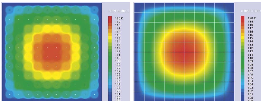
**Figure 4-5.** Detailed model of a Posiva-BWR fuel assembly (left) and homogenized model (right).
