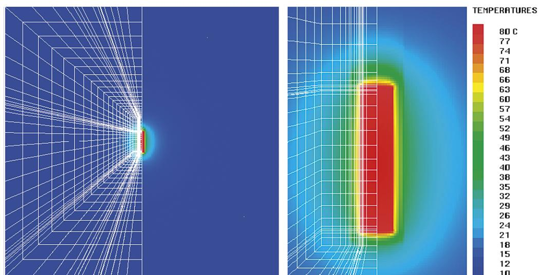
**Figure 6-2.** Example of the mesh and temperature distribution after 1.3 years for a Posiva-BWR model. Left: the whole model. Right: zooming in for the near-field.
