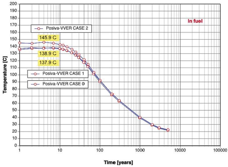
Figure 6-33. Maximum fuel pellet temperature evolution for the Posiva-VVER canister.
