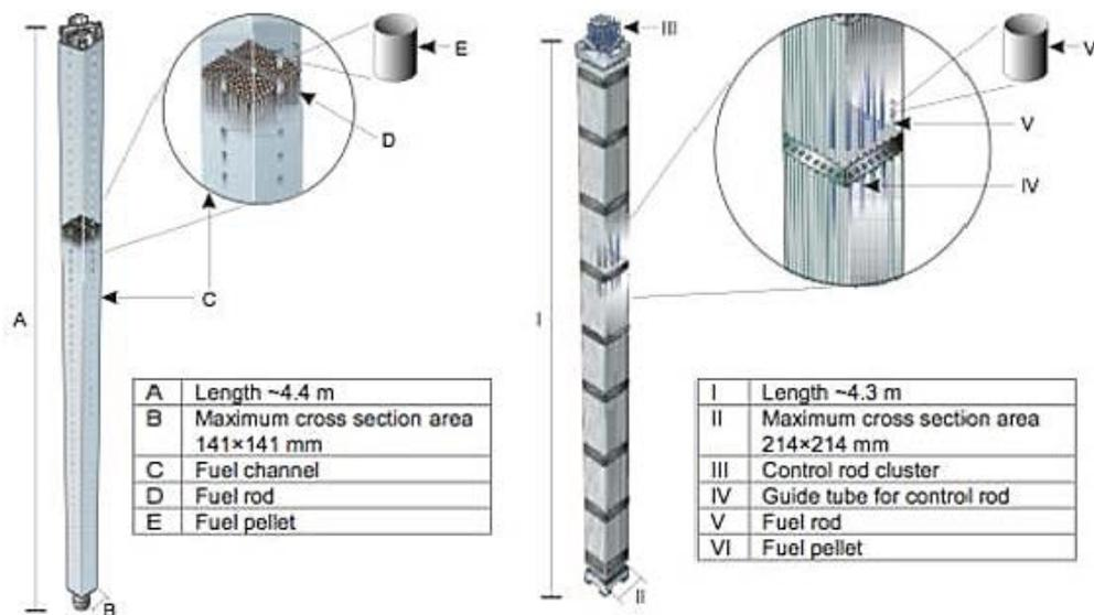
Figure 6-18. SKB-BWR (left) and SKB-PWR fuel assemblies (right) (SKB 2010, Figure 2.5). Data based on specifications provided by the nuclear fuel suppliers.
