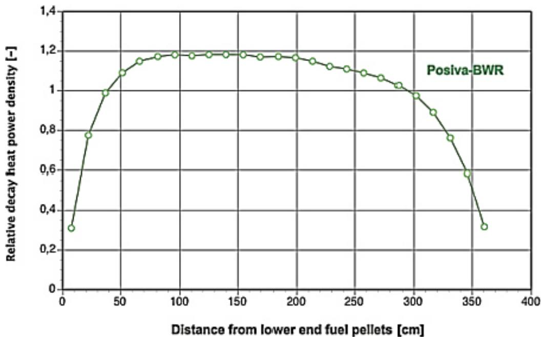
Figure 6-7. Decay heat power density distribution along the BWR fuel assembly length. The active length of the fuel rod is 370 cm.
