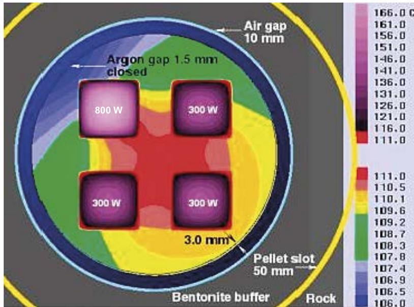
**Figure 7-1.** Asymmetric decay heat power of the SKB-PWR fuel assemblies and the gas gap of 1.5 mm closed near the hottest (800 W) fuel assembly.
