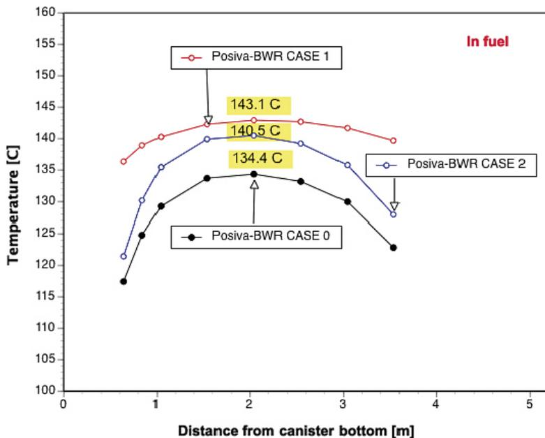
Figure 6-39. Temperature profile of the fuel pellets of the Posiva-BWR canister after 1–4 years.
