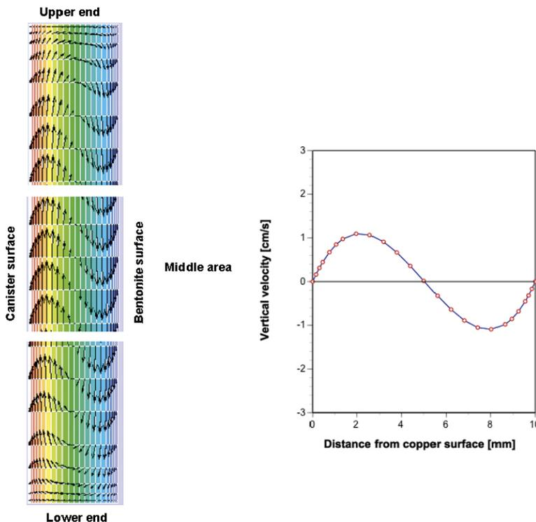
**Figure 7-12.** Natural circulation flow in high, narrow, 10 mm air-filled gap between the canister and the bentonite buffer (left) and the velocity profile at mid-height (right).
