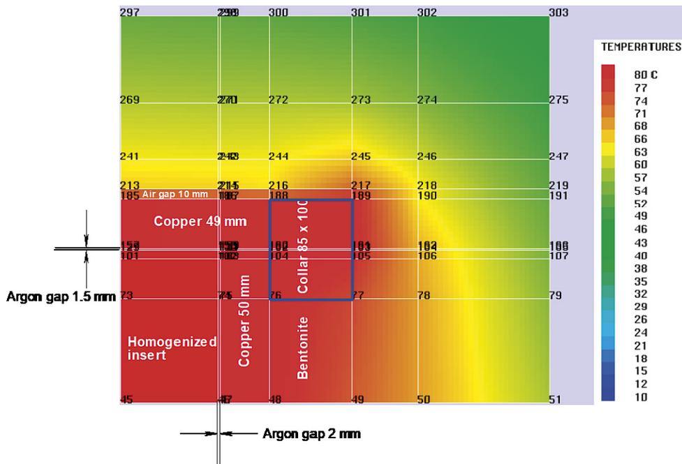
**Figure 6-11.** Temperature distribution in the upper corner of a canister with an 85 mm x 100 mm collar.
