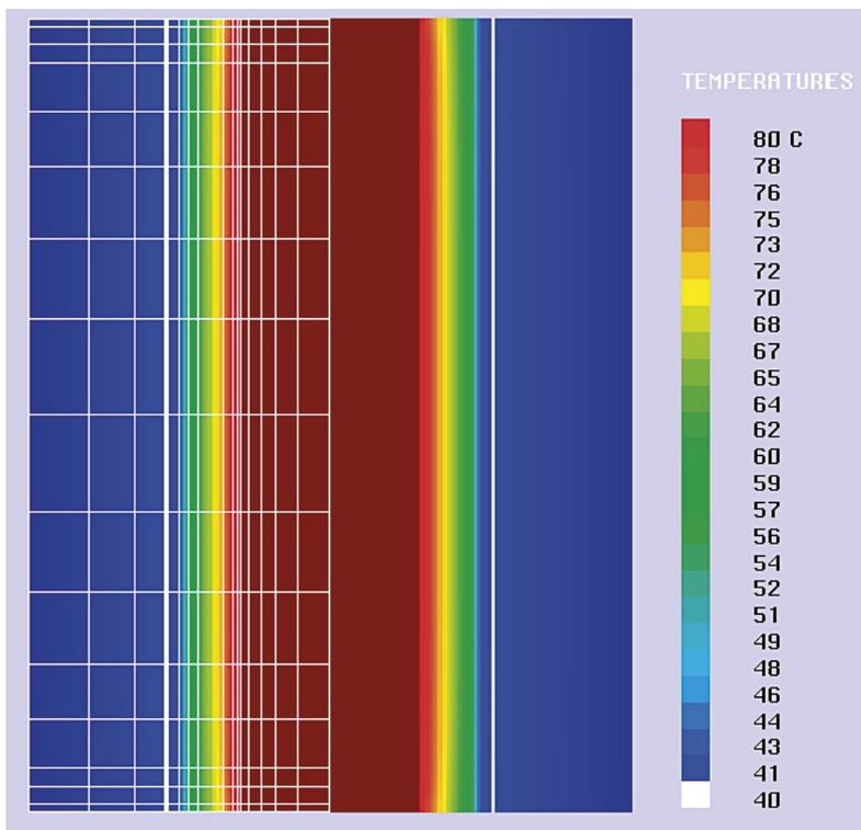
*Figure A-4. A BWR canister is set between two thermally insulated walls.*
