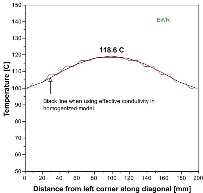
**Figure 4-6.** Temperature distribution along the diagonal at 45 degrees angles starting from the lower-left corner and ending at the upper-right corner and passing through a BWR fuel pellet obtained under a detailed model and under the homogenized model. Temperature on the outer edges is 100 °C.
