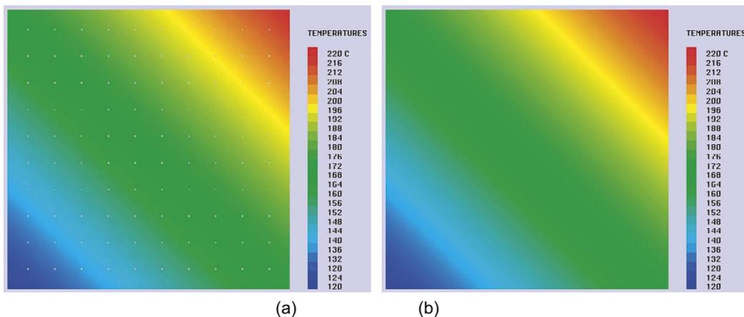
**Figure 4-7.** Temperature distribution in the case where the temperature on the edges changes linearly in the diagonal direction from 120 °C in the lower-left corner to 220 °C in the upper-right corner obtained under a detailed model (a) and under a homogenized model (b).
