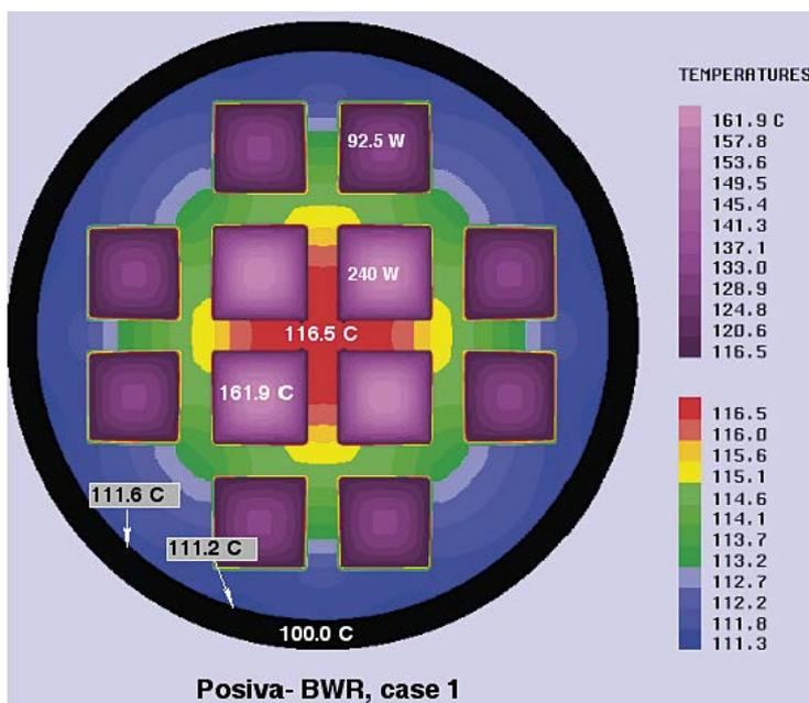
Figure 5-4. Temperatures inside the Posiva-BWR fuel canister in case 1.
