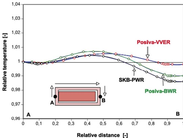
**Figure 6-14.** Relative temperature distribution on the copper surface on the cylindrical part for various canister types. Points A and B are at the centre of the copper shell lids.
