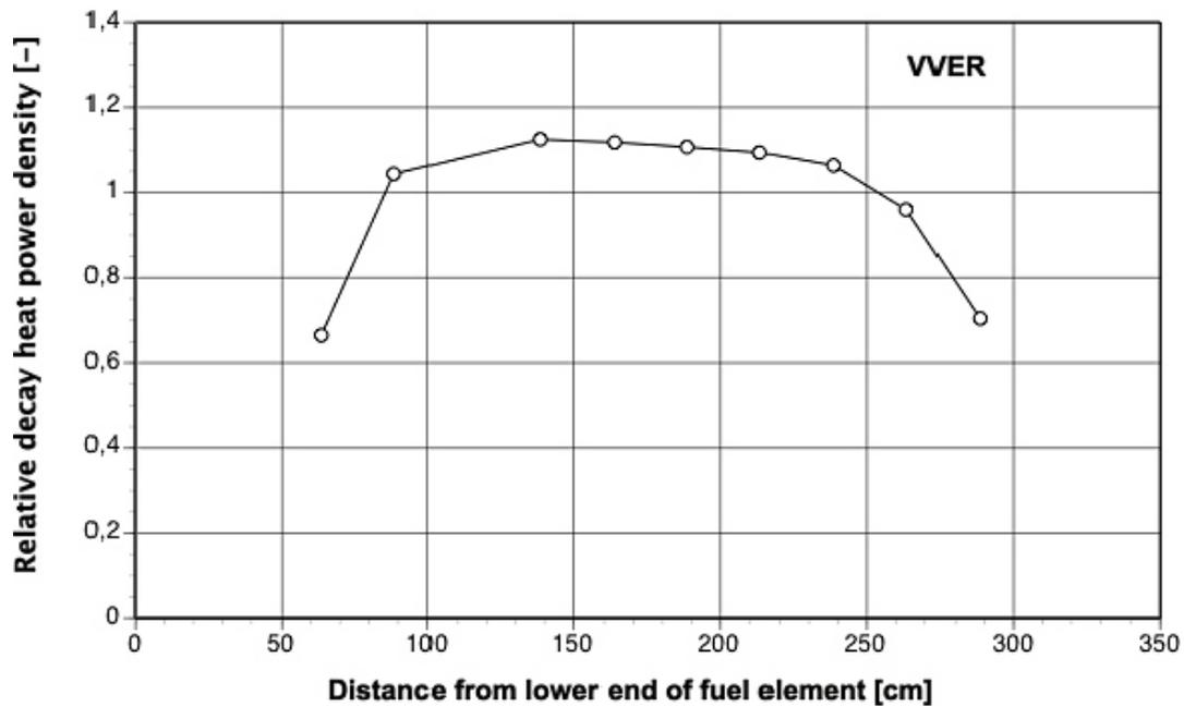
Figure 2-13. Decay heat power density distribution along the Posiva-VVER fuel assembly length. The active length of the fuel rod is 242 cm.
