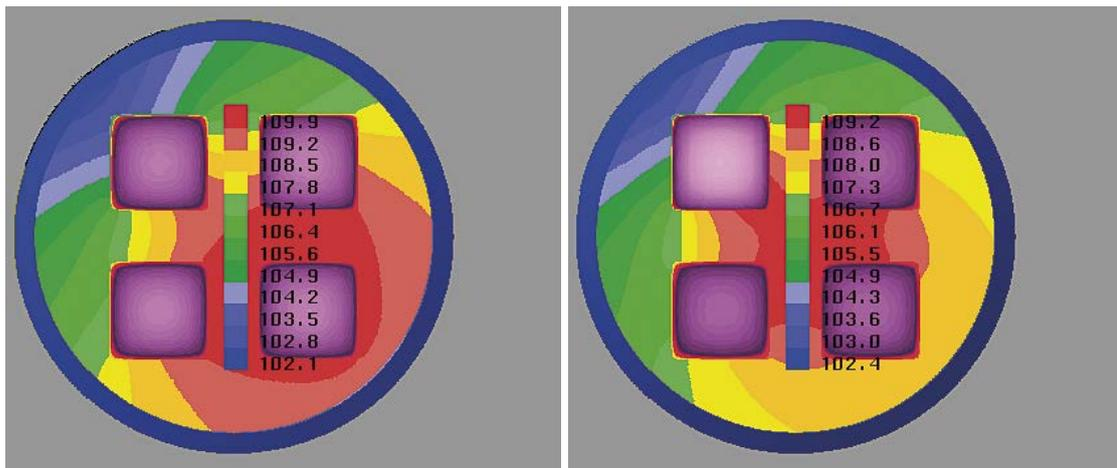
Figure 7-4. Gas gap of 1.5 mm closed with symmetric decay heat powers (left) and asymmetric (right) decay heat power for the SKB-PWR fuel assemblies (right).
