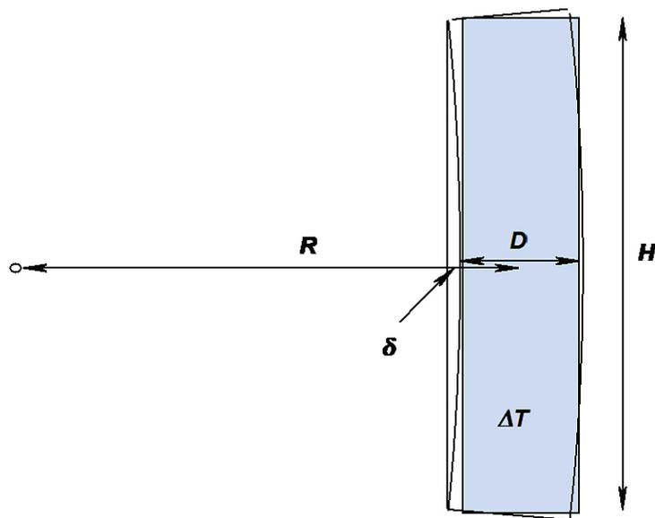
Figure 7-11. Curving of the cast iron insert.
