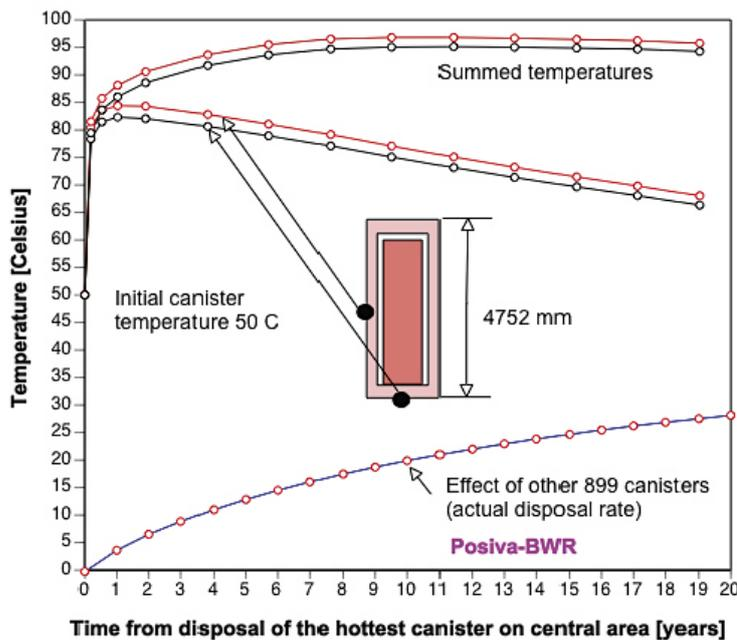
Figure 6-5. Evolution of the maximum temperature in the buffer and in the mid-height of the copper cylinder.
