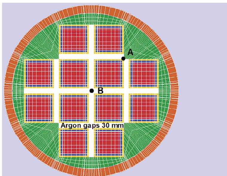
**Figure 7-8.** White colour shows areas in which cast iron does not fill the spaces between the steel channel tubes (Posiva-BWR canister).
