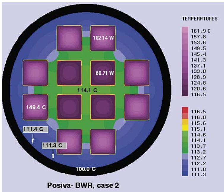
Figure 5-5. Temperatures inside the Posiva-BWR fuel canister in case 2.
