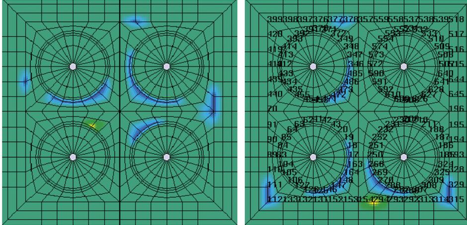
**Figure 3-3.** Demonstration of a view factor determination (the yellow point on a cylinder “sees” the blue areas on other cylinders and fuel channel plates).
