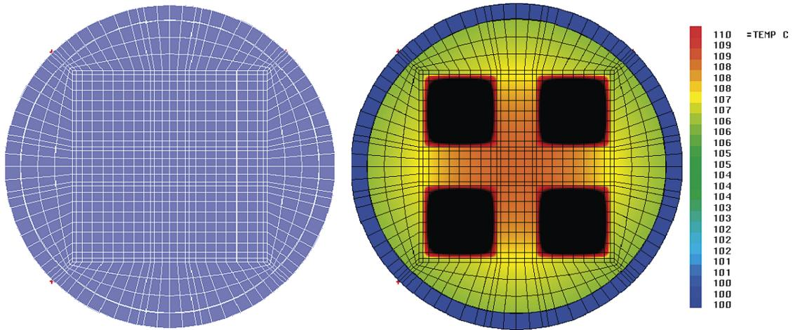
Figure 5-6. Mesh of the homogenized 2D cross-section model of the SKB-PWR fuel canister.
