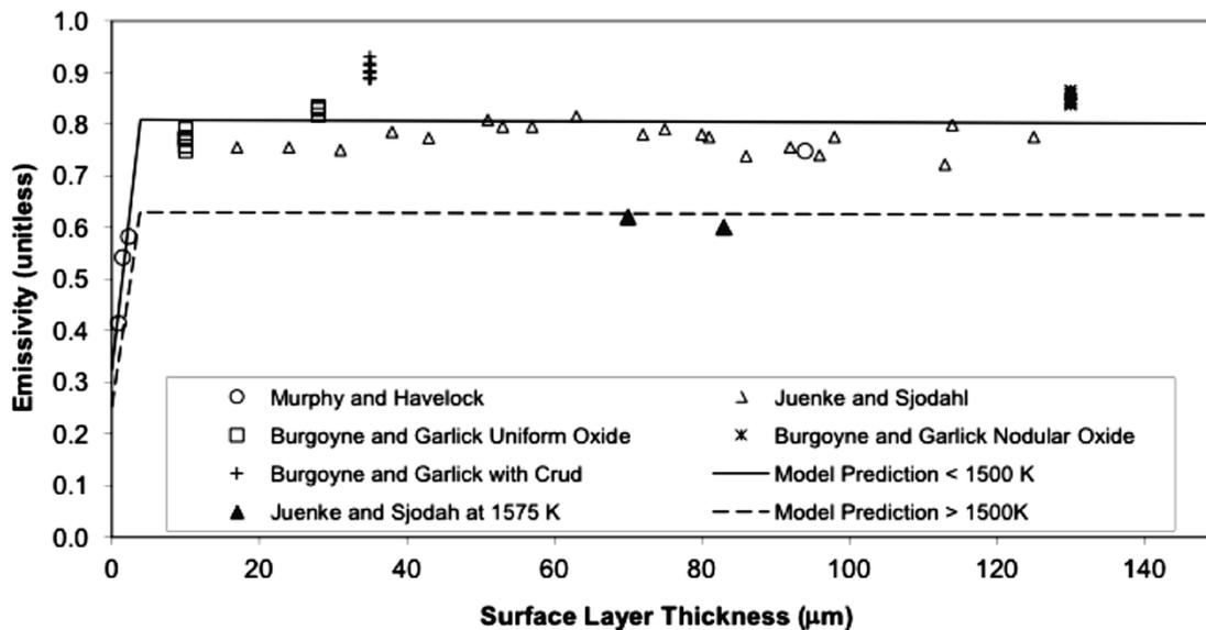
**Figure 2-8.** Model-to-data comparison of cladding oxide emissivity (MATPRO 2014, p 3.13).
