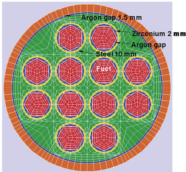
*Figure 5-12. Materials of the homogenized 2D model of the Posiva-VVER fuel canister.*
