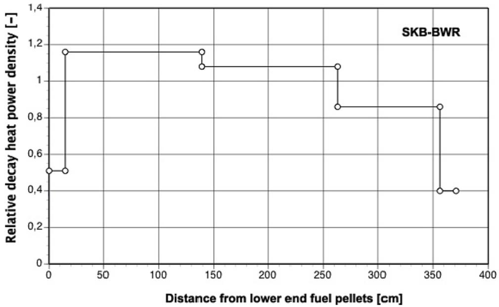
Figure 2-10. Decay heat power density distribution along the SKB-BWR fuel assembly length.
