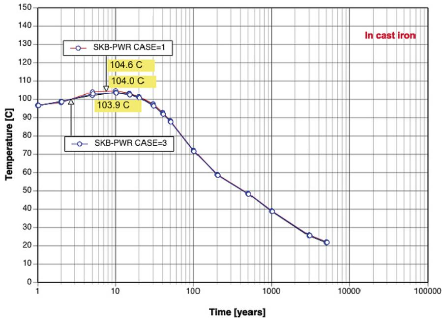
Figure 6-29. Maximum cast iron temperature evolution for the SKB-PWR canister.
