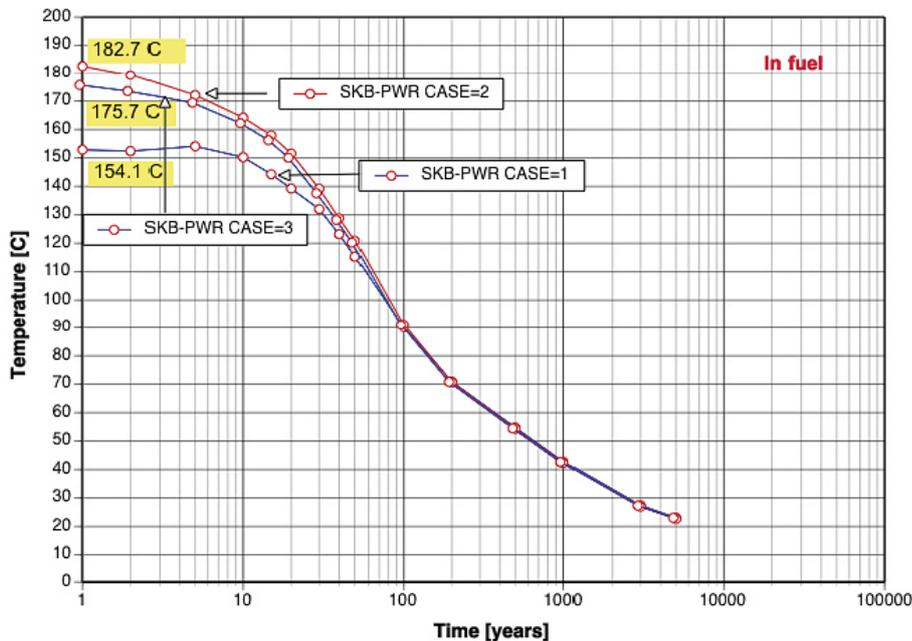
Figure 6-32. Maximum fuel pellet temperature evolution for the SKB-PWR canister.
