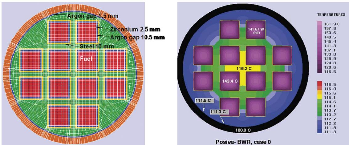
**Figure 6-4.** Materials and gaps in the detailed 2D mesh of the Posiva-BWR fuel canister cross-section (left) and temperature distribution in the Posiva-BWR (0) case (right).
