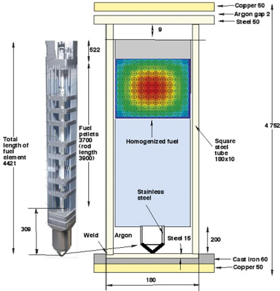
*Figure 6-17. Posiva-BWR-type fuel assembly and surrounding structures in canister (principal drawing, dimensions not to scale). Dimensions according to the Posiva-BWR canister.*
