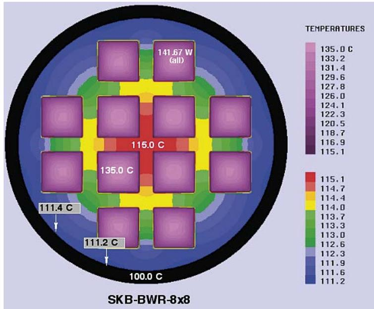
*Figure 5-16. Temperatures inside the SKB-BWR-8 × 8 fuel canister (equal heat powers of 141.67 W in all fuel assemblies).*
