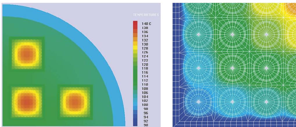
*Figure 4-1. Detailed analysis of the Posiva-BWR canister (Ikonen 2006). The quarter model has approximately 50 000 control volumes.*
