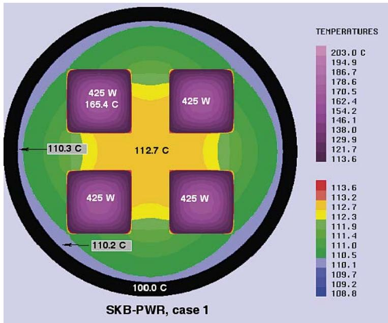
Figure 5-8. Temperatures inside the SKB-PWR fuel canister in case 1.
