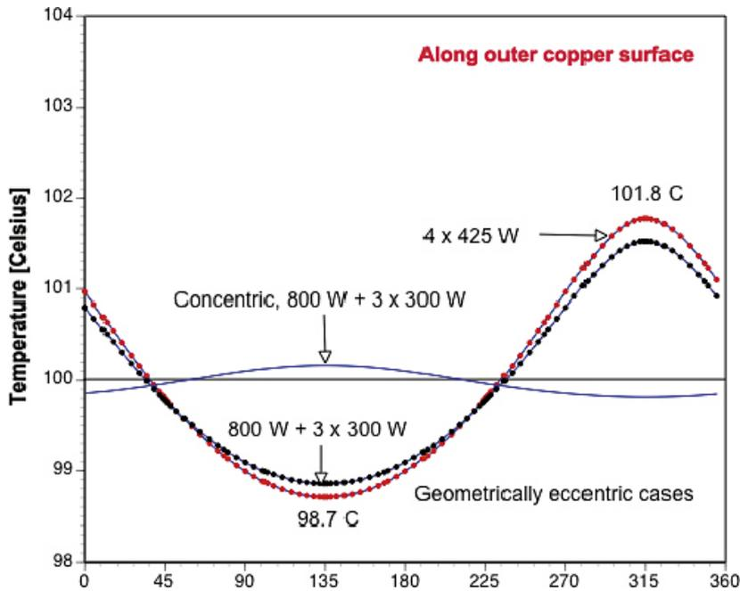
Figure 7-5. Temperature variation in the circumferential direction along the external copper wall when the gap is closed on the opposite side for different cases.
