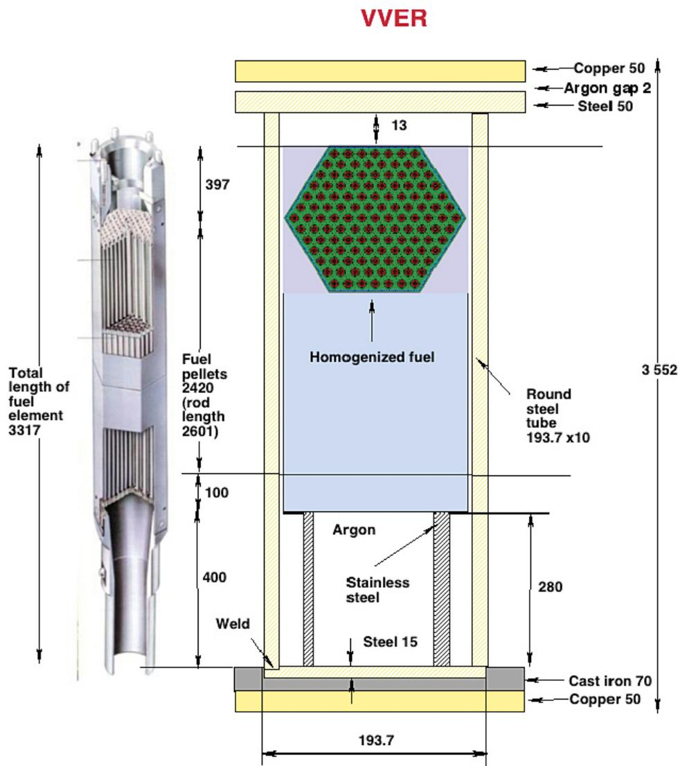
Figure 6-19. VVER-type fuel assembly and surrounding structures in canister (principal drawing, dimensions not to scale).
