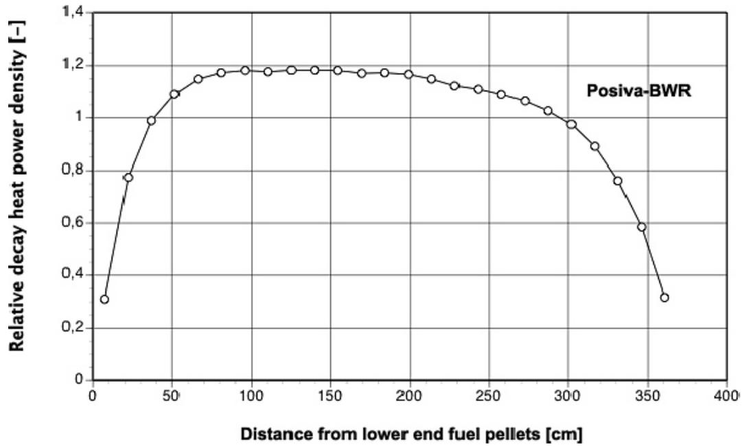
Figure 2-12. Decay heat power density distribution along the Posiva-BWR fuel assembly length. The active length of the fuel rod is 370 cm.
