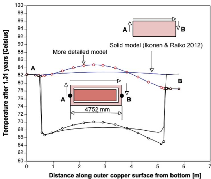
**Figure 6-9.** Temperature distribution along the external surface of a single Posiva-BWR canister after 1.3 years from disposal obtained by the solid homogenous modelling of the whole canister and by the more detailed canister model.
