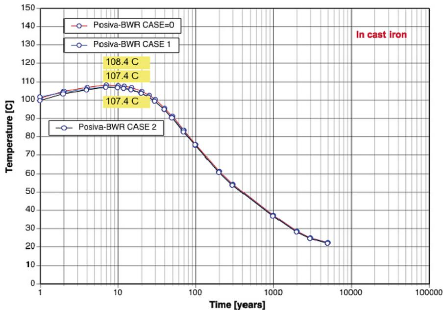
Figure 6-28. Maximum cast iron temperature evolution for the Posiva-BWR canister.
