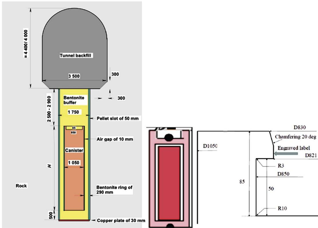
**Figure 6-1.** Nominal dimensions of the disposal hole and tunnel. For the Posiva-BWR type,  $H = 4752$  mm, and for the VVER type,  $H = 3552$  mm. For the SKB canister, the total height is  $H = 4835$  mm due to different bottom end design of the copper shell.
