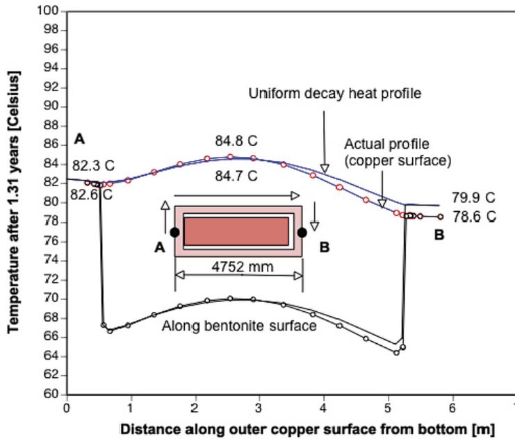
**Figure 6-8.** Temperature distribution along the external surface of a single Posiva-BWR canister with uniform and actual decay heat profiles after 1.3 years from disposal when the maximum temperatures in the bentonite buffer and the copper cylinder are encountered.
