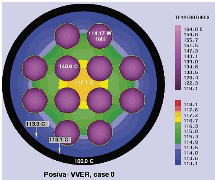
Figure 5-13. Temperatures inside the Posiva-VVER fuel canister in reference case 0.
