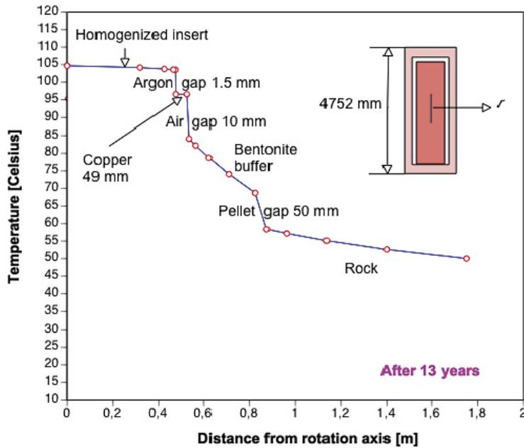
Figure 6-6. Radial temperature distribution of a single Posiva-BWR canister from the rotation axis at the mid-height of the hottest canister after 13 years including also the effect of the other 899 canisters according to Posiva-BWR global repository analysis.
