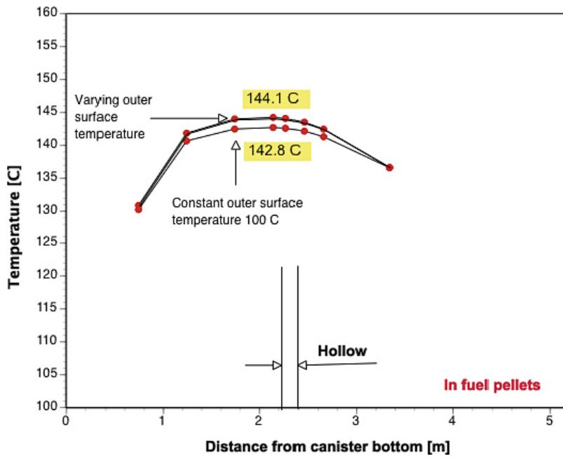
Figure 7-10. Temperature profiles of the fuel pellets of the Posiva-BWR canister with and without a hollow in the cast iron (actual longitudinal decay heat profile).
