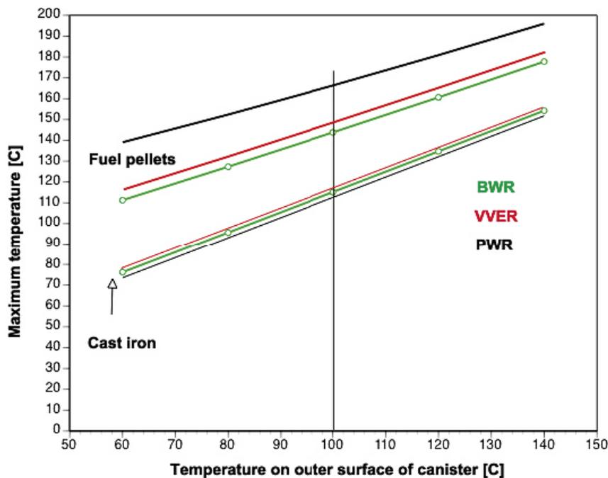
Figure 5-17. Maximum fuel pellet and cast iron temperatures as a function of the canister outer surface temperature.
