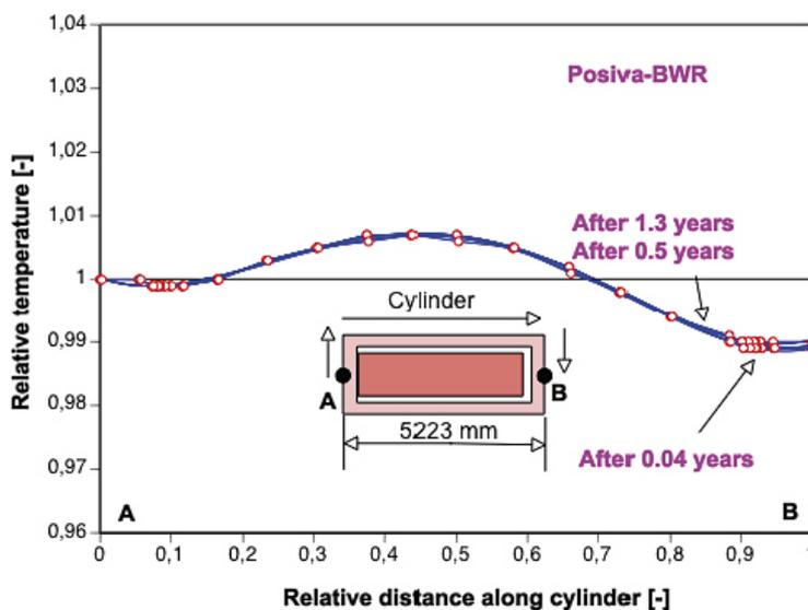
Figure 6-13. Relative temperature distribution on the copper surface starting from the centre of the lower lid and ending at the centre of the upper lid.
