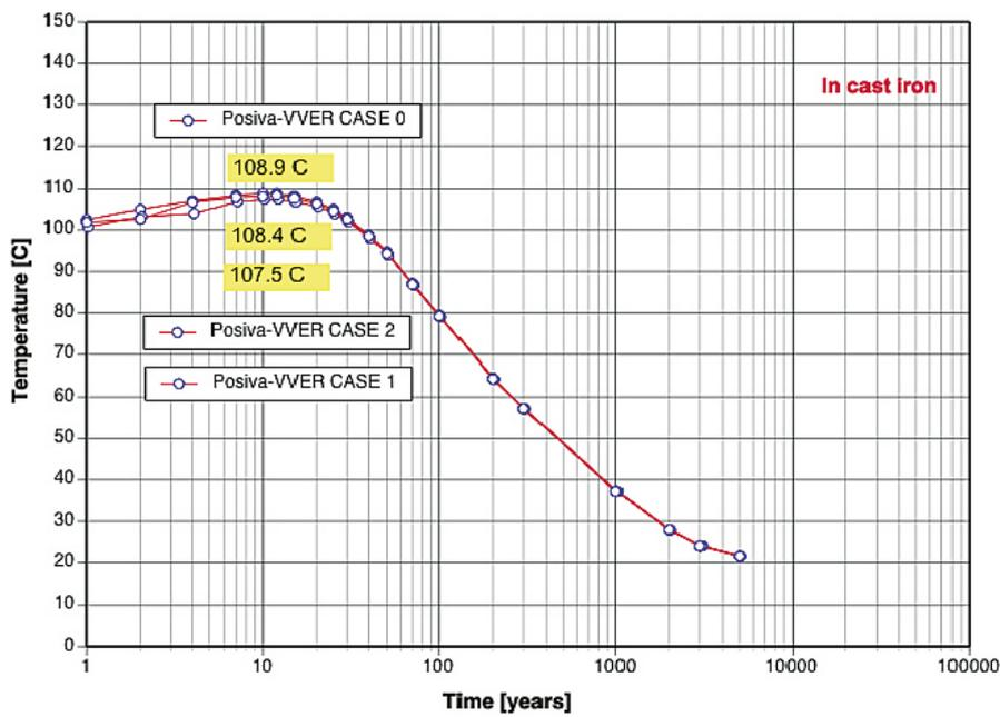
Figure 6-30. Maximum cast iron temperature evolution for the Posiva-VVER canister.
