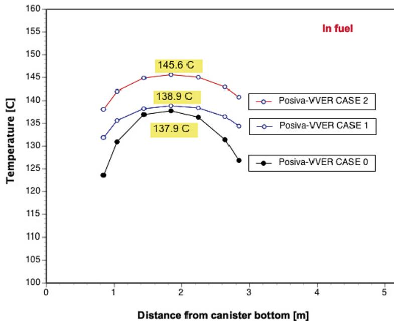
Figure 6-41. Temperature profile of the fuel pellets of the Posiva-VVER canister after 1–4 years.
