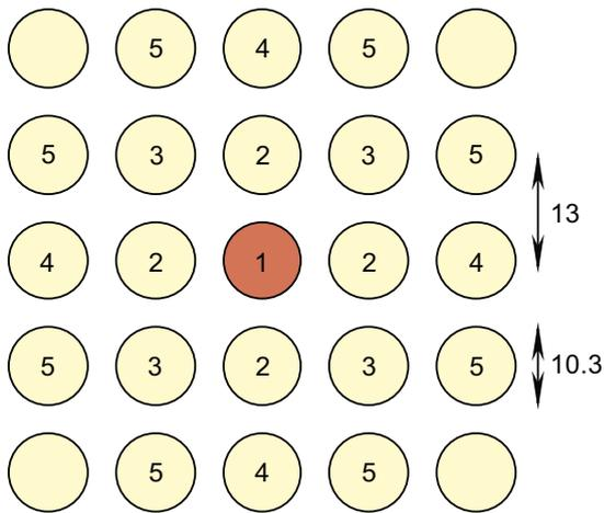
**Figure 4-2.** BWR rods and estimation of the radiation heat effect from neighbouring rods on the rod denoted as “1”.
