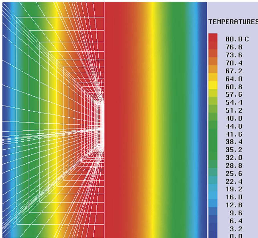
Figure A-3. Uniform heat generation in a homogenous cylinder.
