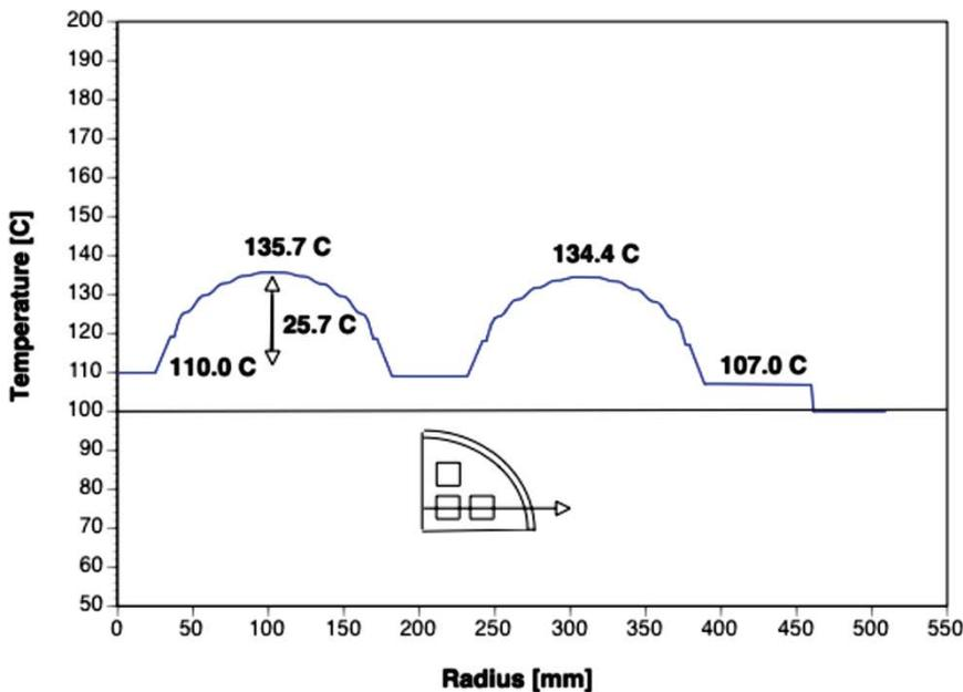
**Figure 4-3.** Temperature distributions along horizontal line passing through the middle point of two fuel assemblies in the Posiva-BWR canister.
