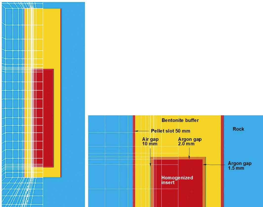
**Figure 6-3.** Material types of the axisymmetric model of the Posiva-BWR fuel canister.
