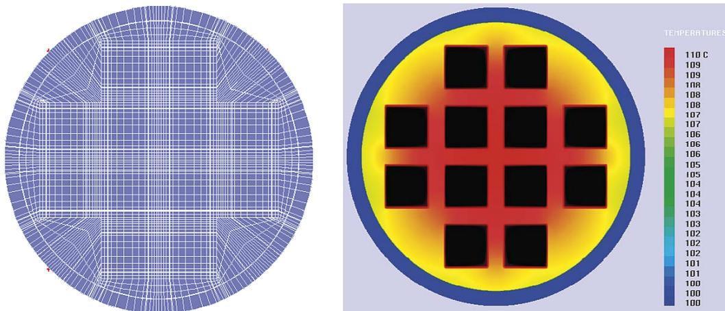
*Figure 5-1. Mesh of the homogenized cross-section 2D model of the Posiva-BWR fuel canister.*
